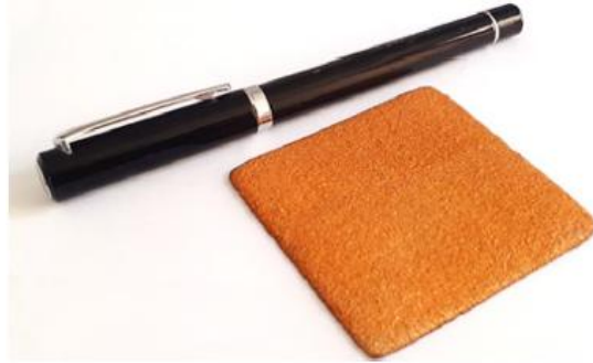
Figure 8. Fabricated three-layer radiation shield sample
