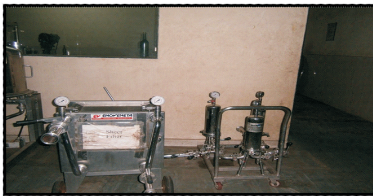
Photo Plate :4. Sheet Filter
