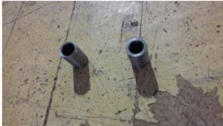
Fig.3 Trunions with internal threading
