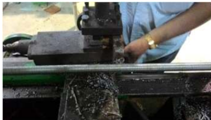
Fig.2 Forming of power screw on lathe
