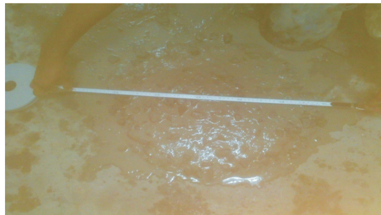
Fig: Slump Flow test in rang of 550-800 mm
