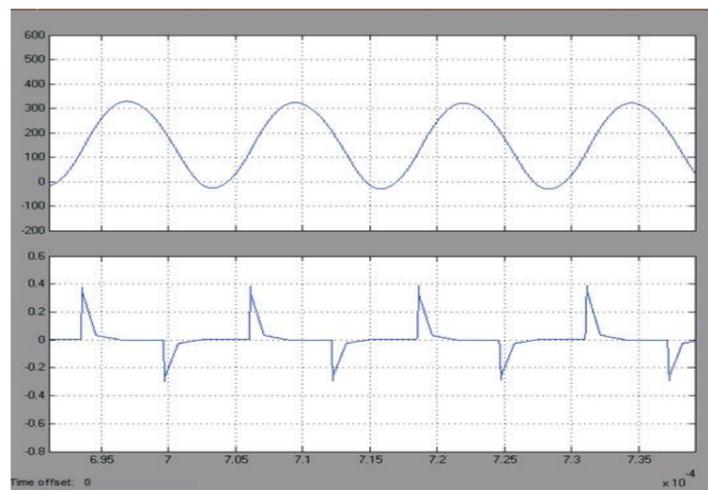
**Fig. 5.3 Simulation output of Resonant voltage and current flowing in the auxiliary circuit.**
