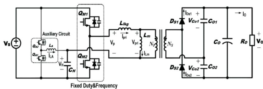
**Fig.2.1 Block diagram of proposed PWM-controlled Quasi Resonant Converter**
