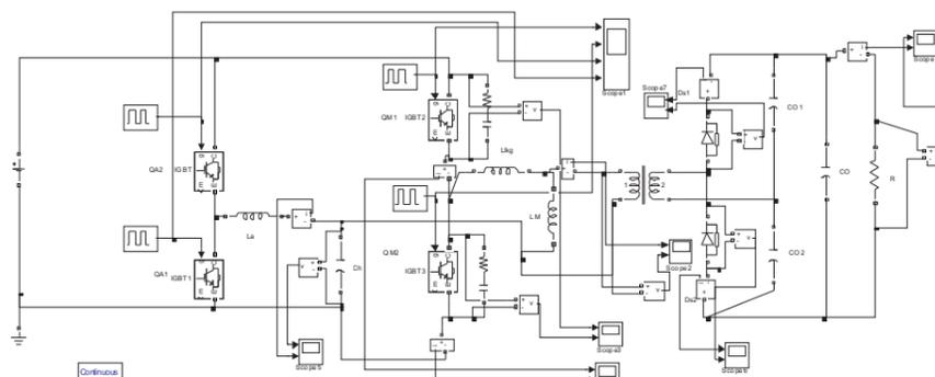
Fig. 5.1 MATLAB Simulink model of the PWM-controlled QRC with R load
