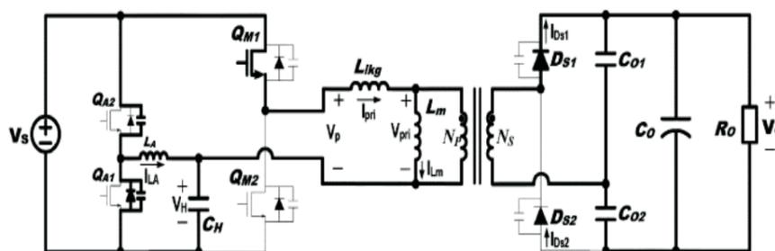
After QA2 is turned off, ILA starts to increase and decrease the phase-node voltage of QA2 and QA1 respectively. When the voltage across QA1 becomes 0V, ILA begins to flow through the internal diode of QA1.
