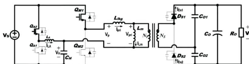
When  $QA_2$  is turned on, mode 2 begins. During this mode, the primary resonant capacitor,  $C_H$ , is additionally charged from the input source,  $V_S$ , through the auxiliary inductor  $L_A$  operating in discontinuous conduction mode (DCM). It is assumed that  $L_A$  is large enough to approximate  $I_{LA}$  which is increased and decreased linearly. The slope of  $I_{LA}$  can be obtained as follows:
