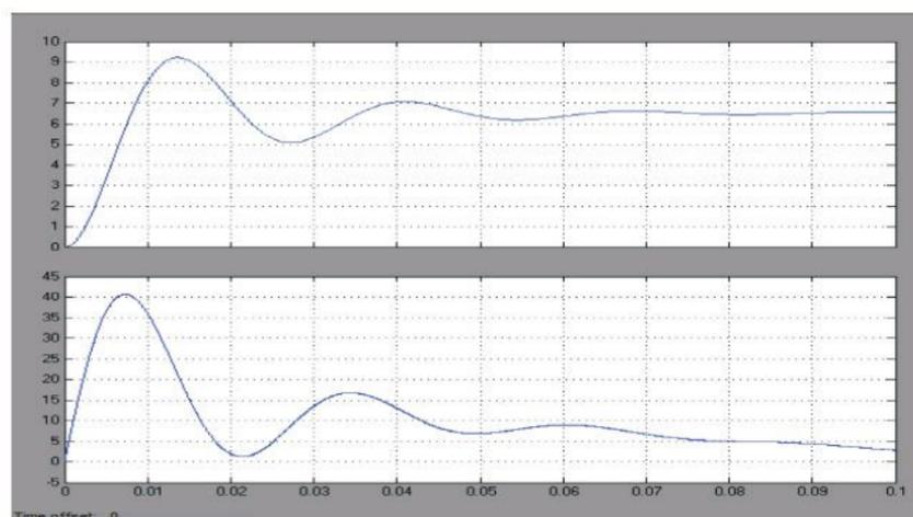
**Fig. 5.6 Simulation output of speed of the dc motor load**
