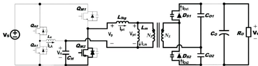
At t<sub>4</sub>, When I<sub>pri</sub> is smaller than I<sub>LM</sub>, the current of the secondary side of the transformer flows oppositely through the junction capacitors, DS1 and DS2. Since the voltage across each diode is increased and decreased respectively, the commutation between DS1 and DS2 is started. During this mode, the ZVS turned on of QM2 can be achieved. After DS2 is fully conducting, mode 5 is finished.
