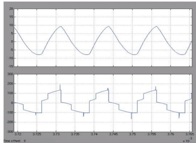
**Fig. 5.2 Simulation output of Current and voltage of the primary side**
