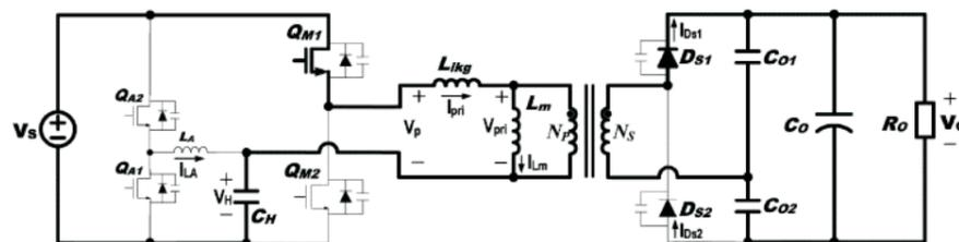
The primary current  $I_{pri}$ , which rises with resonance between the leakage inductor and overall resonant capacitor, is given by
