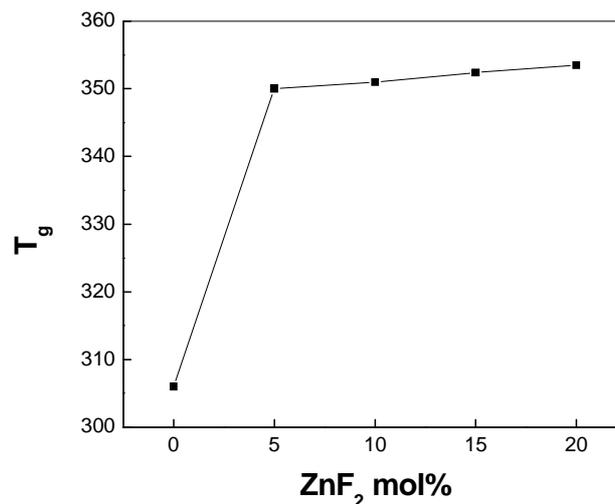
Figure 2 Variation of T<sub>g</sub> with ZnF<sub>2</sub> mol% of Eu-BTZF glasses
