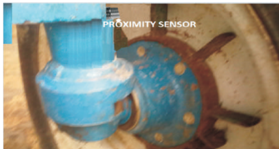
Fig 4 Proximity switch and iron ring fitted on a tractor wheel to measure RPM
