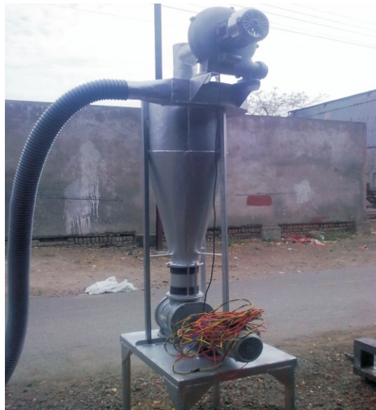
Fig . Pneumatic conveying system
