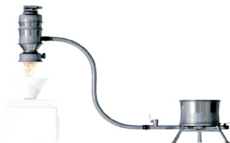
Fig1.1- pneumatic conveying system
