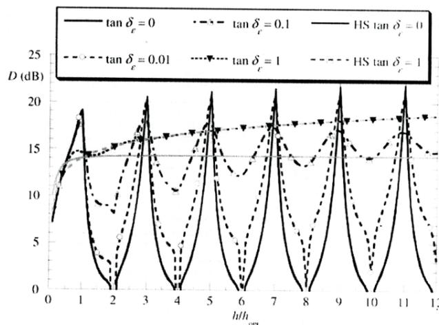
Figure 5 Directivity at broadside [in dB] as a function of the thickness  $h$  for a lossless grounded slab with  $h_s = h/2$ , for different values of the loss tangent. Also shown are results for lossless and lossy half-spaces, where the distance of the source from the interface is the same as for the slab. The optimum thickness  $H_{opt} = 59.2\text{mm}$  is chosen from Eq. (3) when  $f = 1.008\%$  (this corresponds to  $\epsilon_r = 0.0158$ )
